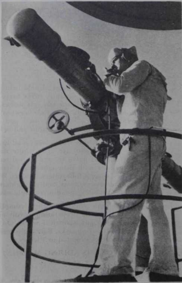
Small range finder. A big one fills a freight car, contains 100 precision optical elements
